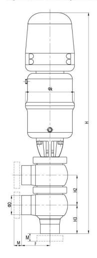
single seat valve with position sensor
